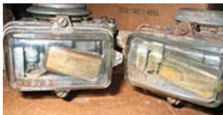
**Figure 3 - Holley "Visi-Flo" model #1904 carburetors from the 1950s, factory equipped with transparent glass bowls**
