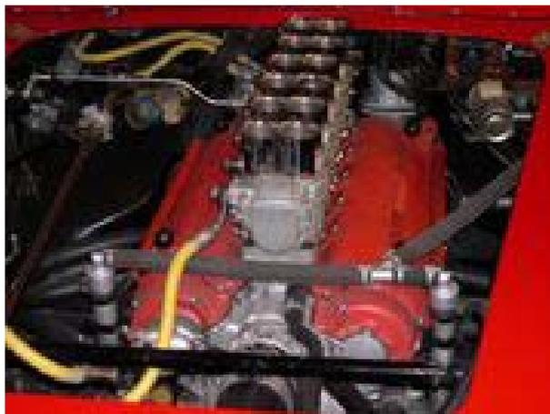
**Figure 5 - Colombo Type 125 "Testa Rossa" engine in a 1961 Ferrari 250TR Spyder with six Weber two-barrel carburetors inducing air through 12 air horns; one individually adjustable barrel for each cylinder.**
