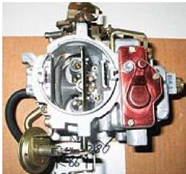
Figure 4 - Holley model #2280 2-barrel carburettor
