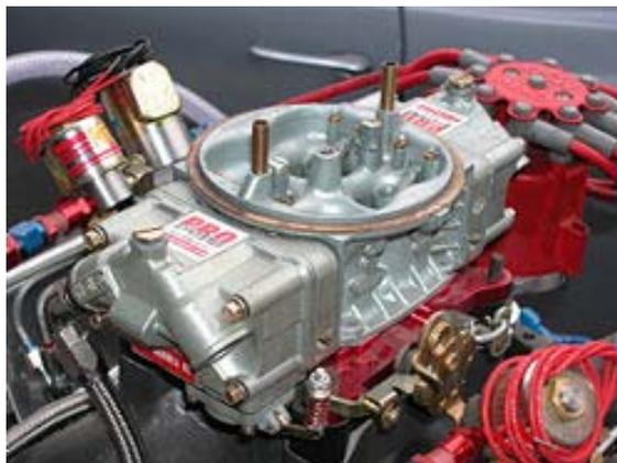
Figure 1 - A high performance 4-barrel carburettor
